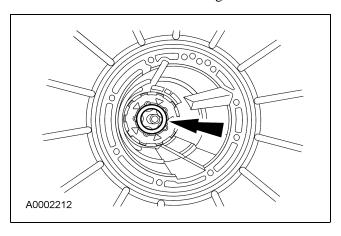
29. Install the spacer on the input shell, using petroleum jelly to hold it in place.
